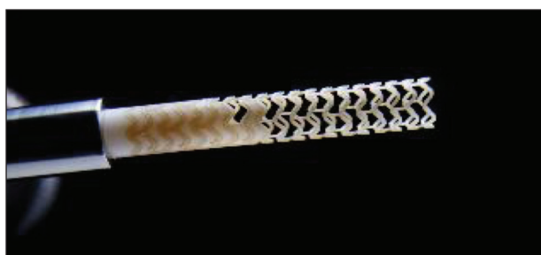
Figure 2. Laser-cutting of Fantom from a Tyrocore tube.
